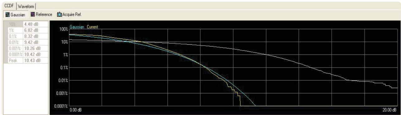
Figure 11. Waveform CCDF calculates the CCDF and peak-to-average ratio using the entire LTE-TDD waveform (with downlink signal off and uplink signal on)
